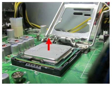
**IMPORTANT:** If you are going to install a new processor, note the arrow on the corner to make sure the processor is properly oriented over the socket.
